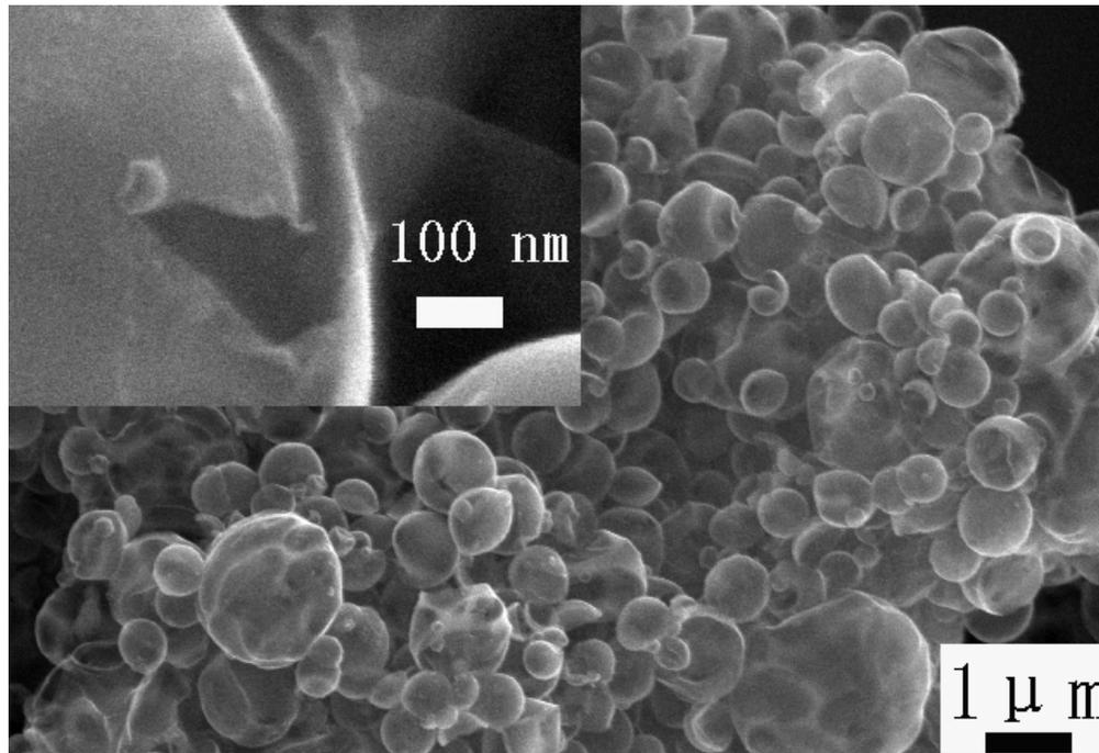
**SEM images** of carbon hollow spheres obtained by USP of sodium citrate aqueous solutions
