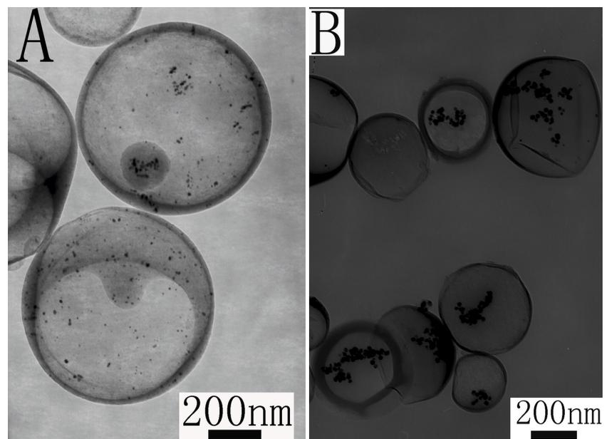
**XRD and TEM** of (A) Pt@carbon and (B) Ag@Carbon obtained via USP of aqueous solutions containing metal salts and sodium citrate
