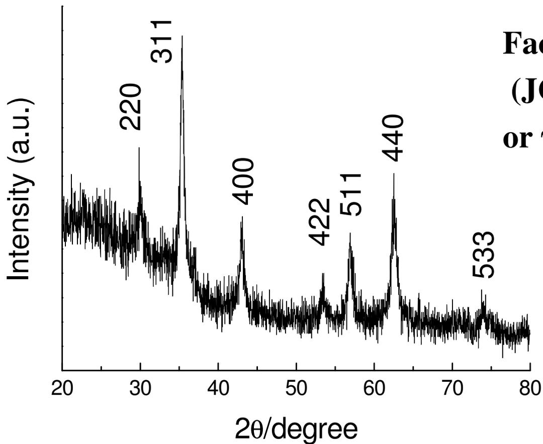
**Face-centered cubic  $\text{Fe}_3\text{O}_4$**
