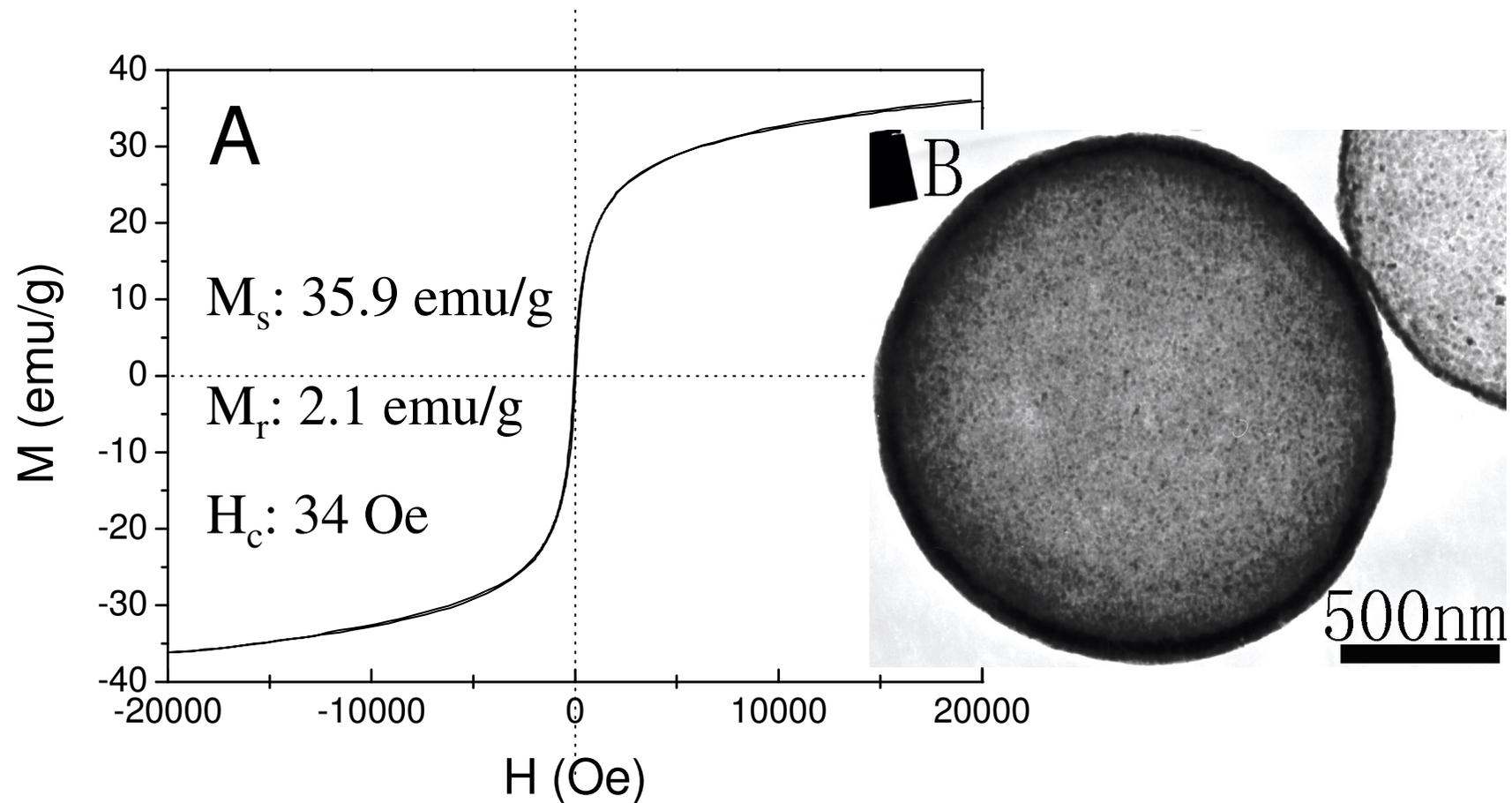
(A) The **M–H hysteresis loop** and (B) **TEM image** of MCHMs after acid treatment (pH = 1) at room temperature for 10 d.
