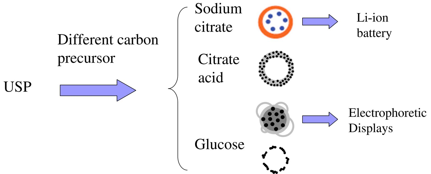
**Schematic** of the ultrasonic spray pyrolysis (USP) synthesis of nanocomposites
