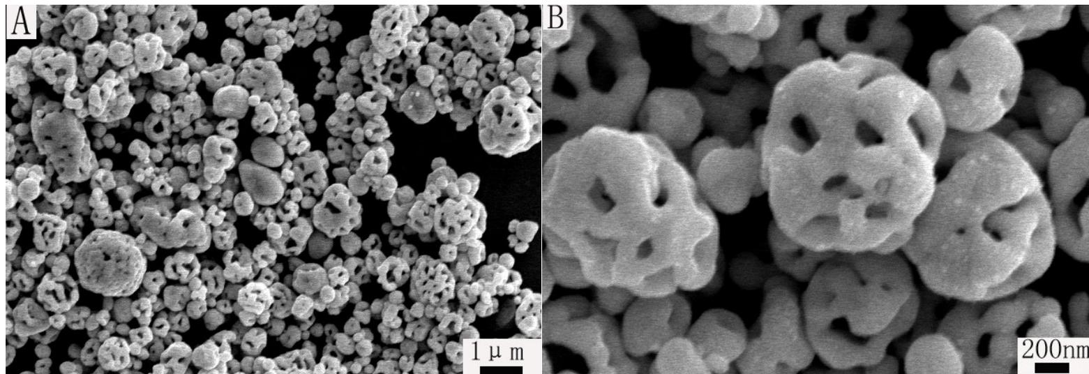
SEM of SPHS prepared via USP of aqueous solutions containing glucose and  $\text{AgNO}_3$
