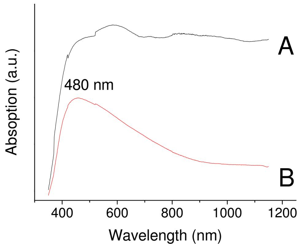
**Vis-NIR spectrum** of SPHS (A) and silver solid spheres (B) fabricated via USP.
