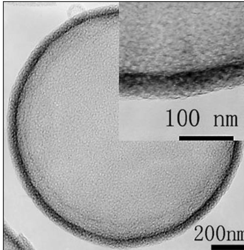
**TEM images** of porous hollow carbon spheres obtained by acid treatment of  $\text{Fe}_3\text{O}_4\text{-C}$  magnetic hollow spheres in concentrated HCl (12 M) for 12 h.
