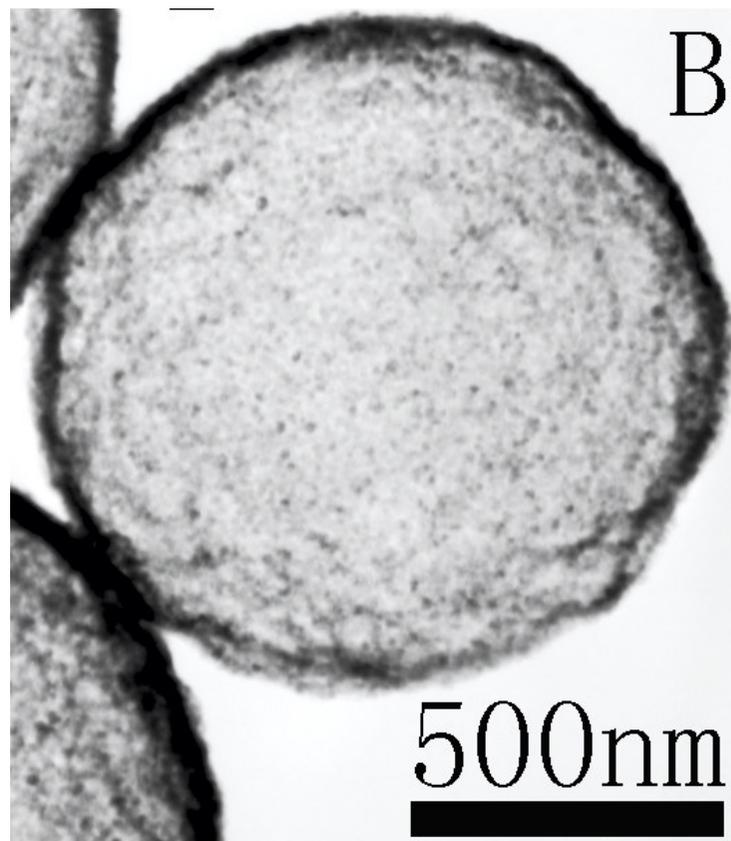
**TEM images** of  $\text{Fe}_3\text{O}_4\text{-C}$  magnetic hollow spheres obtained by USP of aqueous solutions containing  $\text{FeCl}_2$  and citrate acid
