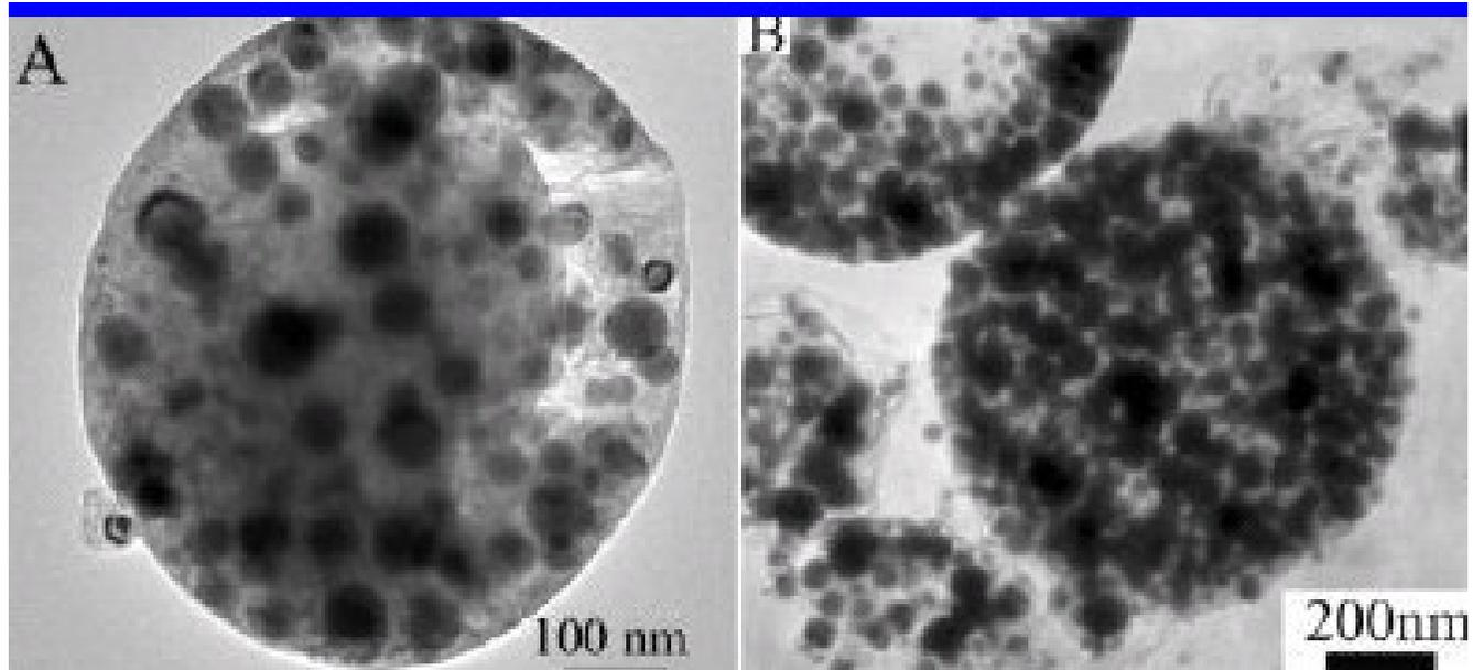
**TEM images** of Sn@carbon solids (A) collected without water at 700 °C and (B) collected with water at 500 °C.
