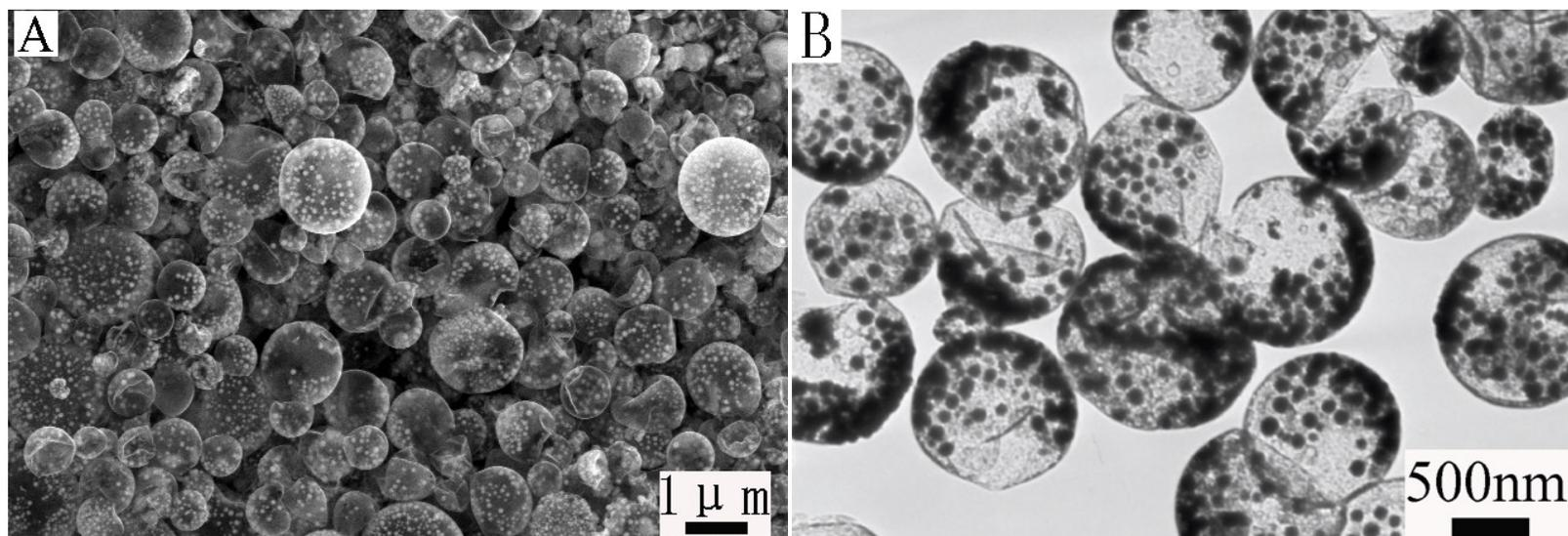
**SEM and TEM** images of Sn@carbon obtained via USP of aqueous solutions containing  $\text{SnCl}_4$  and sodium citrate
