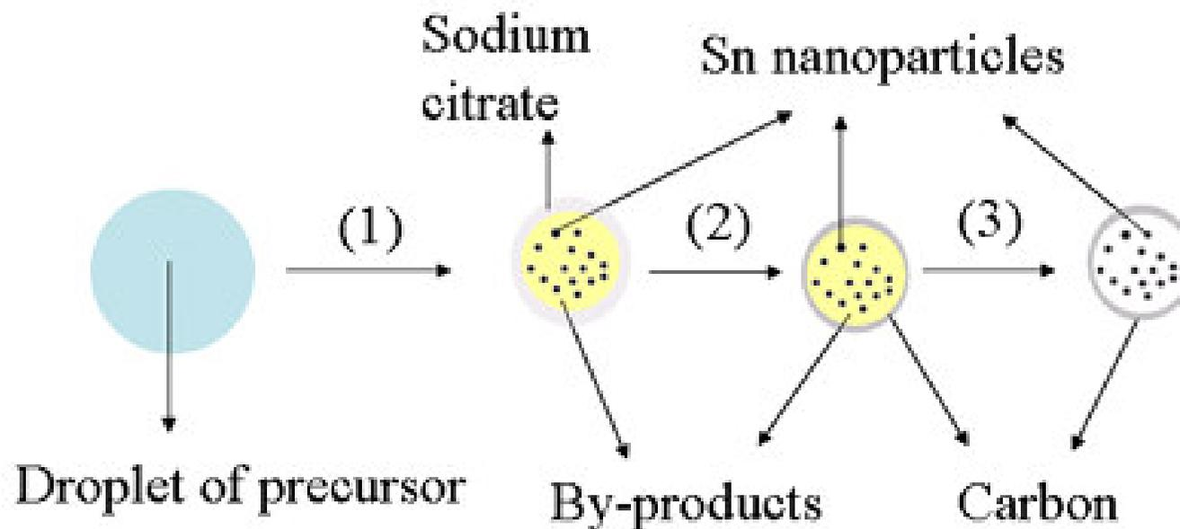
**Illustration** of the M@carbon obtained via USP of aqueous solutions containing metal salts and sodium citrate
