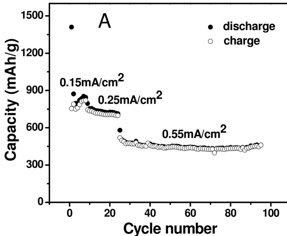
The cycling performance in the 0 mV-3 V (vs. Li<sup>+</sup>/Li) voltage window at different rate of Sn@carbon (46 wt % Sn).
