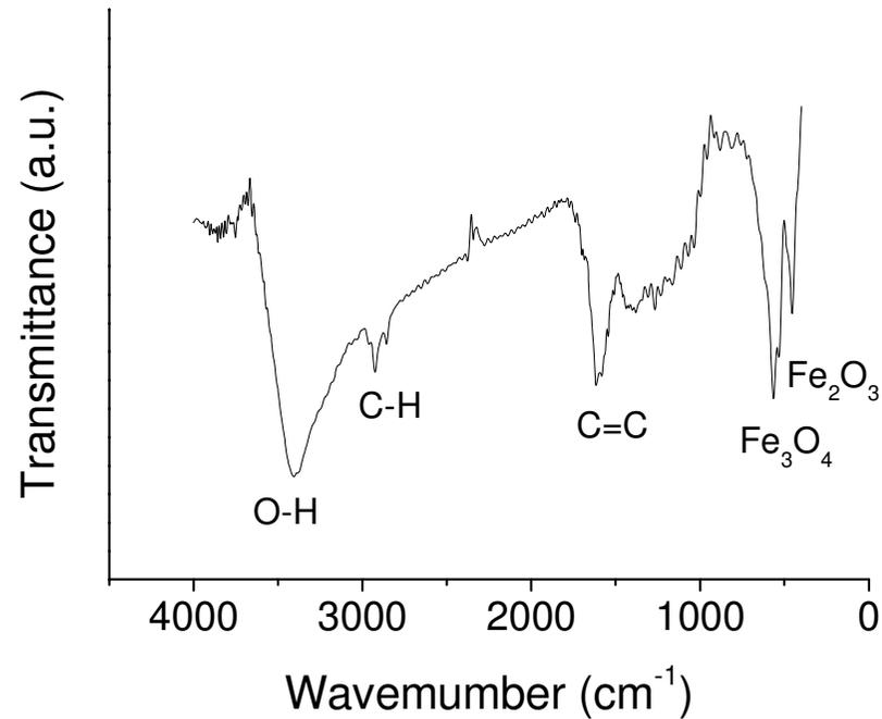
FT-IR spectrum of carbon-iron oxide
