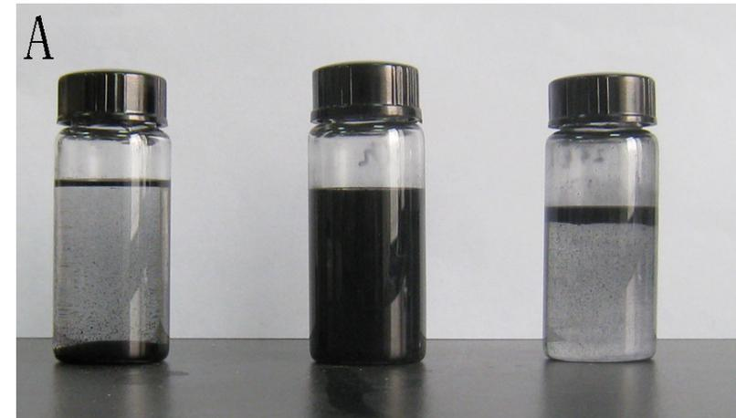
Carbon-iron oxide with (from left to right 0, 1, 12 h) etching time are dispersed in tetrachloroethylene.
