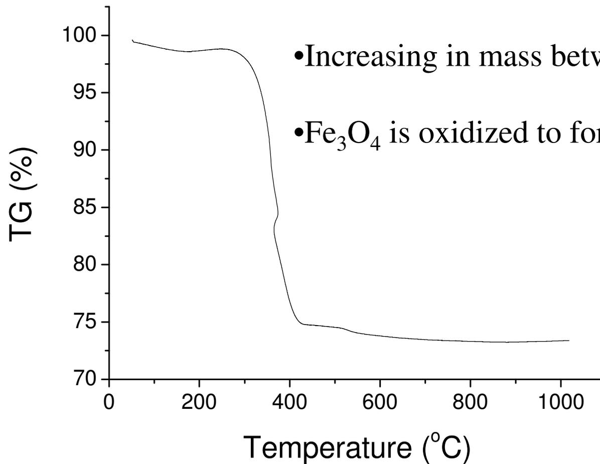
**TGA** of Fe<sub>3</sub>O<sub>4</sub>-C magnetic hollow spheres
