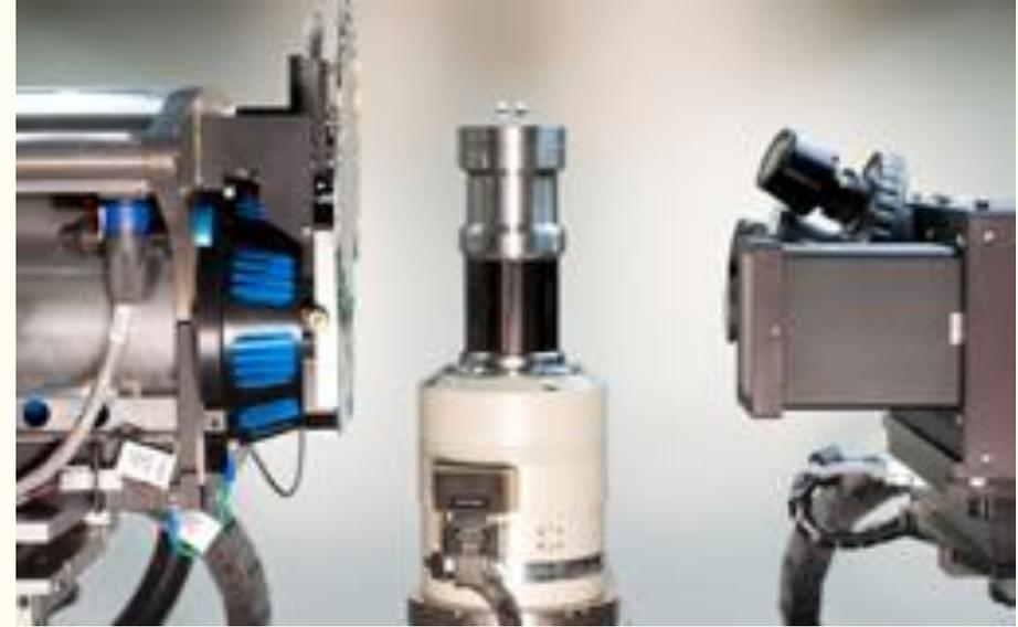
The inside of a Zeiss Xradia Versa X-ray Laboratory Microscope
