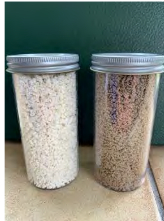
50% OCC/ 50% kaolin mineral/ MFC composite (right) and control with NBSK
