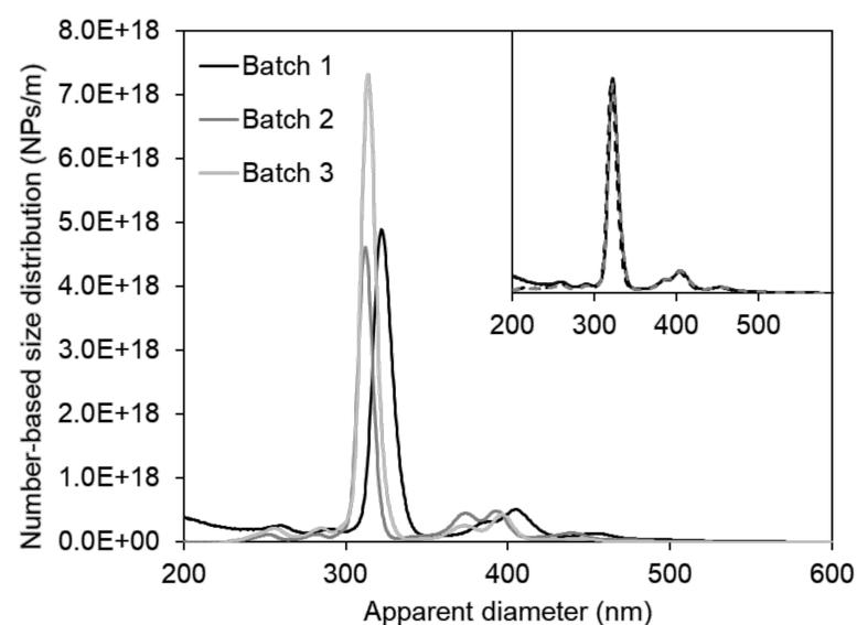
Figure 1: Particle size distribution determined by DCS, showing low variability between batches of SonoTran Particles. Insert: Variability between aliquots of Batch 1.
