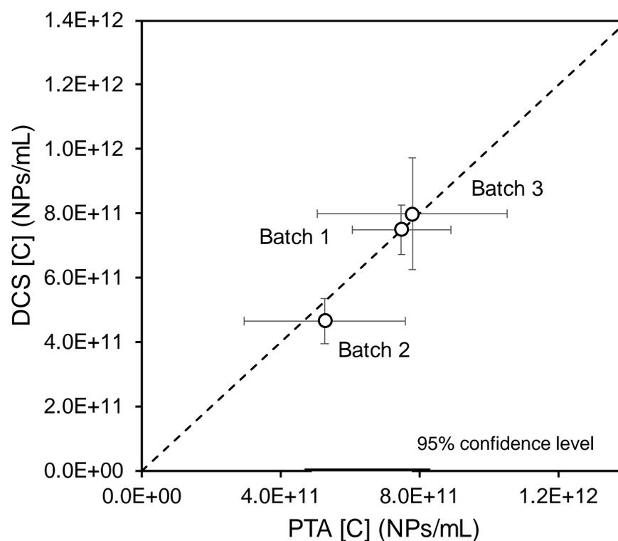
Figure 3: Particle number concentration of the SonoTran Particle batches as measured by the calibrated DCS method and PTA. Error bars show method repeatability with a 95% confidence level. The dash line shows the identity relationship.
