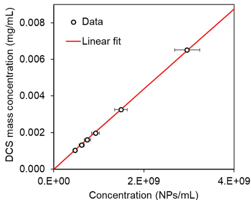
Figure 2: Calibration curve for concentration measurements performed by DCS. The X-axis shows the particle number concentration from PTA and dilution factors, the Y-axis shows the mass concentration measured by DCS by integrating the weight-based size distribution.
