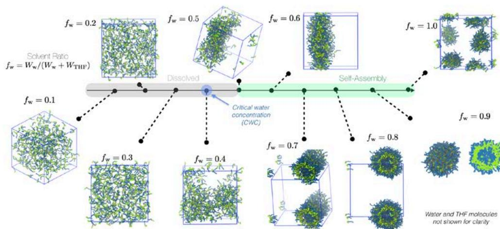
**Figure 1.** Morphological phase diagram of PEO6-b-PBMA4 at 10wt% in mixtures of water and THF for different solvent ratio ( $f_w$ ). In the simulation snapshots the PBMA and PEO blocks correspond to green and blue beads, respectively.
