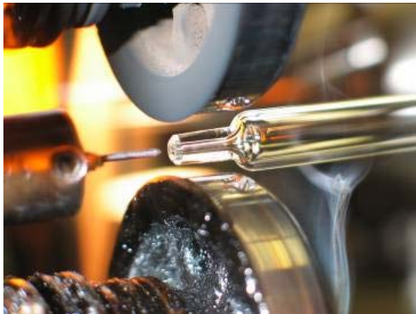
Channel Forming of Staked Needle Syringe with Tungsten Pin
