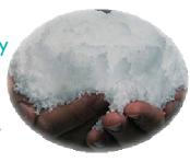
Instant Snow Polymer is made by cross-linking molecules of the sodium polyacrylate polymer. When water is added, the individual clusters internally hydrate and expand, forming small, fluffy clusters that do not cling to surrounding clusters. This appears as a powdery snow. When more water is added, the water molecules hydrate the external surface of these clusters, and the clusters begin to adhere to one another. This appears as slush.
