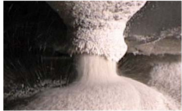
Sand adhered to a hopper
