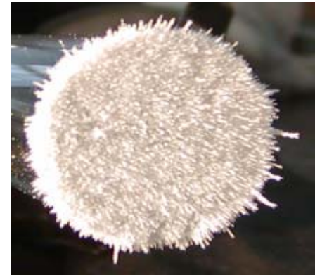
Cellulose adhered to a charged rod
