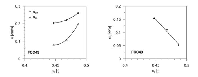
As expected, the tensile strenght of the bulk decreases along with its bulk density.
