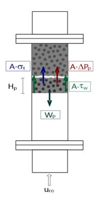
At  $u_{ro}$  the tensile strenght  $s_t$  resists 'raining' even if the pressure drop across the plug is lower than its weight of per unit section:
