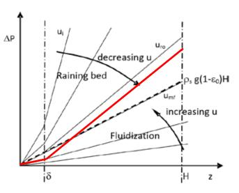
The presence of the cohesive force makes possible to the drag force decrease **under the value of the buoyant weight** per unit surface up to the fall of a plug.
