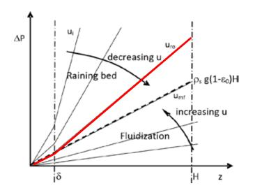
An equilibrium is established between drag and gravity at the external layer of the bed.
