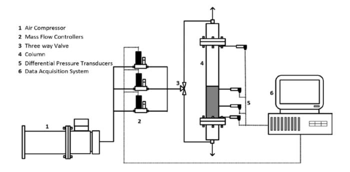
Column diameter: 54 mm Column height: 400 mm
